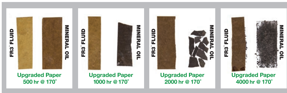
Insulation aging study comparing thermally upgraded paper using FR3 fluid vs. mineral oil.
