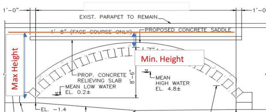
Assume Excavation Depth =  $2/3 * \text{max height} * 1/3 \text{ min height}$
