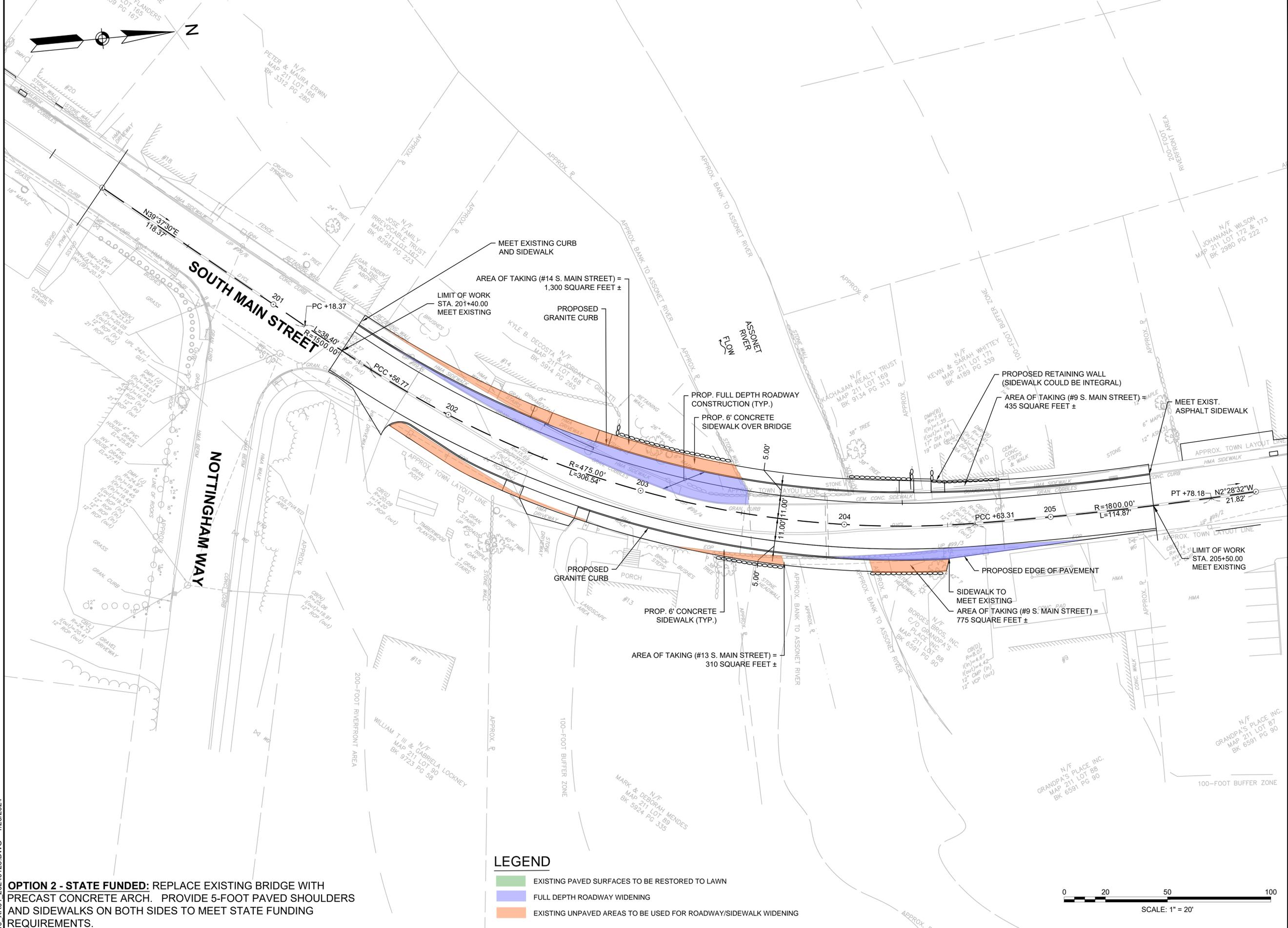
**OPTION 2 - STATE FUNDED:** REPLACE EXISTING BRIDGE WITH PRECAST CONCRETE ARCH. PROVIDE 5-FOOT PAVED SHOULDERS AND SIDEWALKS ON BOTH SIDES TO MEET STATE FUNDING REQUIREMENTS.
