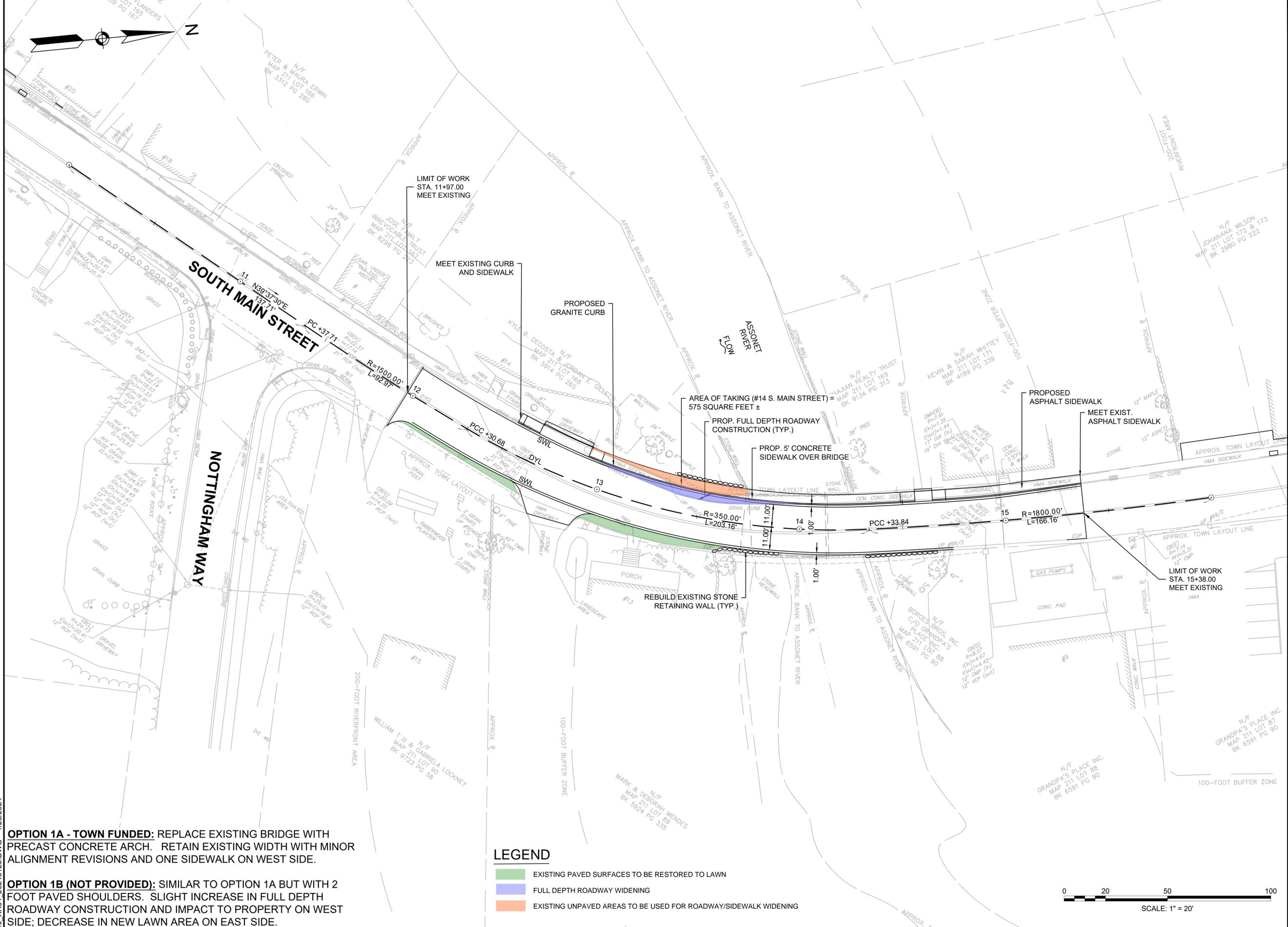
**OPTION 1A - TOWN FUNDED:** REPLACE EXISTING BRIDGE WITH PRECAST CONCRETE ARCH. RETAIN EXISTING WIDTH WITH MINOR ALIGNMENT REVISIONS AND ONE SIDEWALK ON WEST SIDE.
