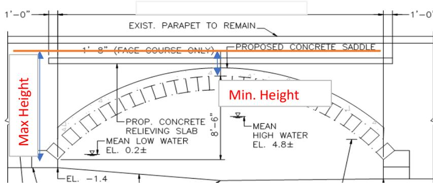
Assume Excavation Depth =  $\frac{2}{3} * \text{max height} * \frac{1}{3} \text{ min height}$
